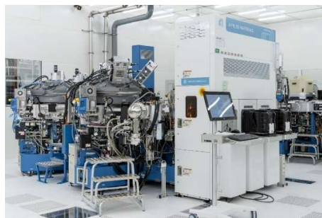
Fig. 1: 300mm wafer-level PVD tool for MTJ stack deposition.
